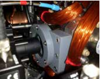
3D printed piece (grey) custom made with the printer to hold a magnet and allow a viewport
