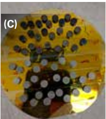
(A) Thermoelectric rings post spin-on doping process (B) Microscopic view of the n and p legs before metallization (C) Thermoelectric wafers mounted for the sputtering step
